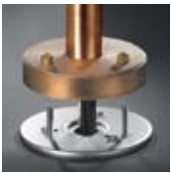
The garden luminaires on this double page have a die cast bronze base plate. A stainless steel mounting plate is bolted to a matching anchorage unit made of galvanized steel or to a foundation.
