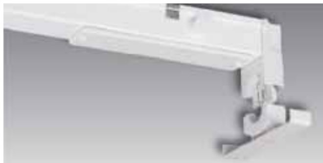
Cover plate 185 and push-fit lampholder combined in a captive unit. Retaining strap: Aids first-time installation and when changing lamps, not suited for continuous duty!
