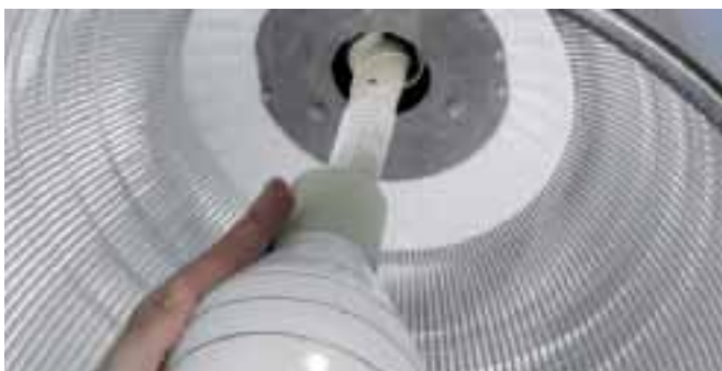
Induction lamp, energy transmission without an electrical connection.
