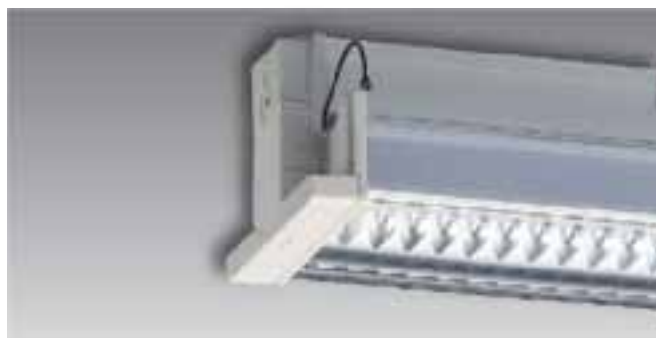
Easy mounting of cover and FL with built-in mirrored dark-light louver. Retaining strap: Aids first-time installation and when changing lamps, not suited for continuous duty!
