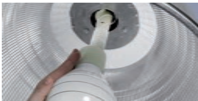
induction illuminant, energy transfer without electrical connection
