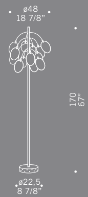
PRO•SECCO R12 12x20W-12V G4 alogeno bispina halogen bi-pin
