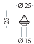
Terminale in plastica per tubo Ø 20x2 Plastic tube top end finial Ø 20x2
