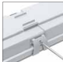
Technopolymer wide dimension cover clips distribute the loading force for a good seal and ease of operation (6x18W, 10x36W and 12x58W). Clips are lockable using anti-tamper screw accessory (A0412).
